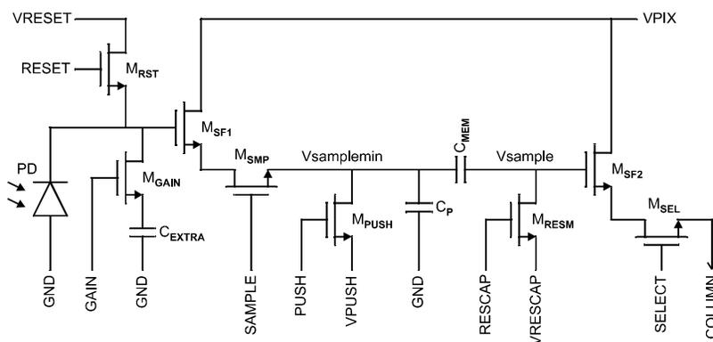
Fig. 4 7T (8T) pixel design
