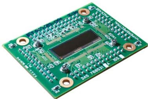
Fig. 6 Packaged Hyperspectral Imager
