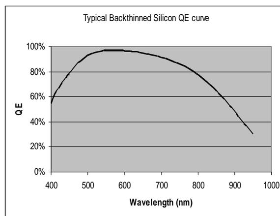
Fig.3. Typical Back-thinned Silicon QE curve.
