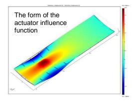
Fig. 1. FEA model of actuator influence function
