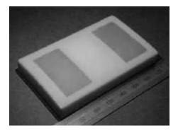
Fig. 5. PZT actuators on former
