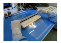
Fig. 7. Glue layer being applied to back of optic
