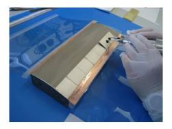
Fig. 9. Placement of actuators on optic
