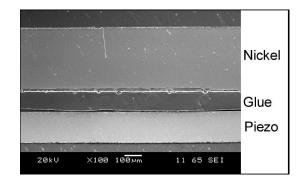
Fig. 8. Cross section of test piece showing glue layer
