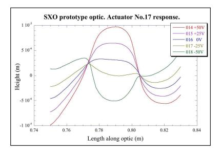
Fig. 11. Long trace profiler measurement of a single actuator at various voltages
