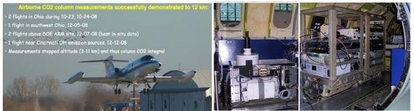
Fig. 1 (left) The NASA Glenn Lear-25 carrying our airborne precursor CO2 lidar instrument during December 2008. (right) Photograph of the interior of the Lear aircraft showing the fall 2008 version of the instrument, with (left to right) the receiver telescope assembly, the laser and electro-optics rack and the electronics/computer rack.
