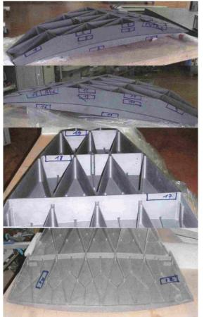
Fig. 9. SiC samples to be cut out from a Herschel M1 spare segment
