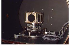
Fig. 7. Circular SiC reference mirror and rectangular samples are mounted on a rotating wheel and placed inside the thermal vacuum chamber
