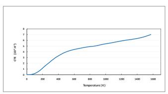
Fig.1. Thermal Expansion of Boostec® SiC versus Temperature
