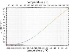
Fig.3. Accurate CTE measurement of Boostec® SiC from [10]
