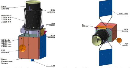
Fig. 4. Geo-Oculus spacecraft configuration (left: stowed, right: deployed) Proc. of SPIE Vol. 10565 105651V-3
