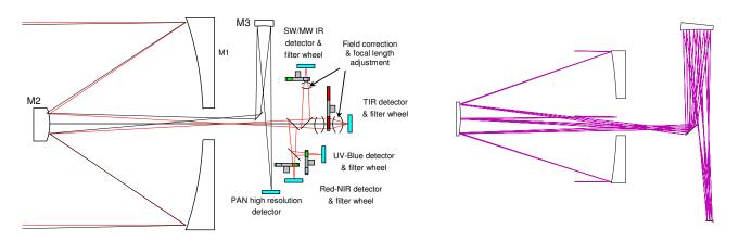
Fig. 6. Optical configuration (left: synoptic, right: PAN channel) Proc. of SPIE Vol. 10565 105651V-4
