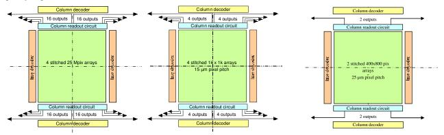
Fig. 7. Detectors architecture (left: UV-VNIR CMOS, middle SWIR/MWIR HgCdTe, right TIR QWIP)
