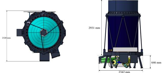
Fig. 8. Instrument mechanical layout Proc. of SPIE Vol. 10565 105651V-6
