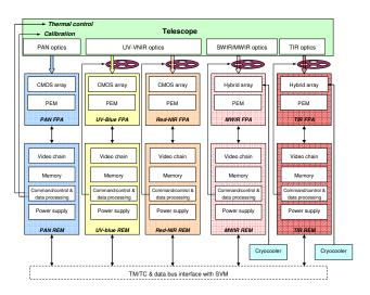
Fig. 9. Electrical architecture of the instrument
