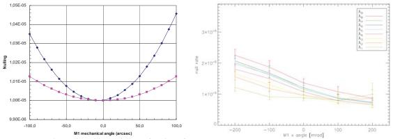
**Fig. 10a:** monochromatic nulling ratio as a function of M1 tilt, with afocals (blue curve) or not (pink curve).
