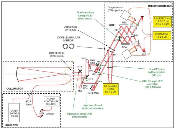
Fig. 1: general setup of PERSEE in its final operational state.
