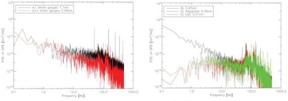
Fig. 5a: OPD residual noise, open loop.
