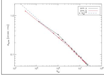
Fig. 4: tip/tilt noise as function of flux (closed loop).
