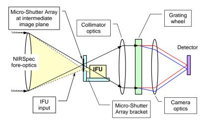
Fig. 1. Schematic of the NIRSpec instrument as relevant to the IFU
