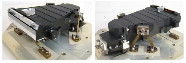
Fig. 5. The flight model IFU assembly (left: front view, right: rear view)
