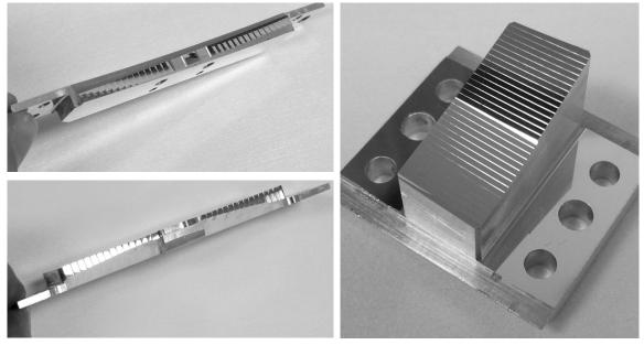
**Fig. 4.** The mirror arrays (clockwise, from right: slicer; slits; pupils with relay 2 at the centre) The slicer has an active area around 25 x 12.5mm, and the long arrays an active length around 75mm.
