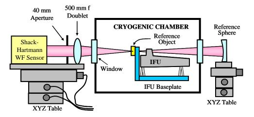
Fig. 6. The principal optical test set-up used in cryogenic tests
