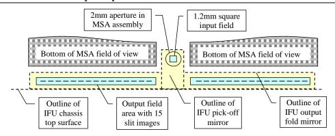
Fig. 2. Schematic of the input and output geometry for the IFU fields of view (not to scale)
