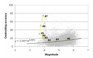
**Fig 9** Centroïding as a function of magnitude (for LCMS based camera in MABS) (#n indicates the number of detector pixels which are saturated in a 4 x 4 interpolation frame) Proc. of SPIE Vol. 10565 1056529-6
