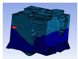
Fig 6 Fundamental eigen-frequency of housing at 1350 Hz
