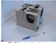
Fig 5 Cast aluminium housing Proc. of SPIE Vol. 10565 1056529-4
