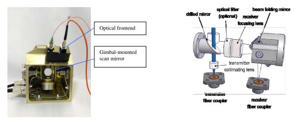
Fig. 3a) RVS ILT sensor head
