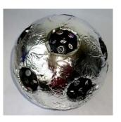
Fig. 1a) Test target sphere containing 12 RR arrays
