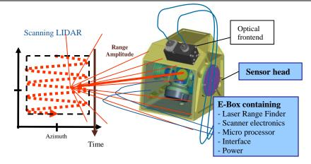
Fig. 2. RVS ILT sensor principle
