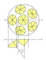
**b**) Geometry of 1 of the retro reflector arrays
