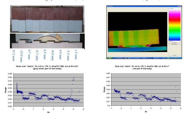
Fig. 5 Test sample and test result for 3D measurement of a non-cooperative target
