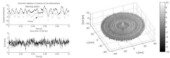
Fig. 4. Noise level at standstill, and typical repeatability for Ø100 mm tilted flat
