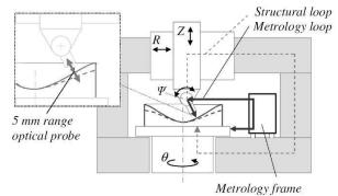
Fig. 2. Machine concept
