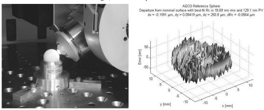
Fig. 5. Measurement result of an Al<sub>2</sub>O<sub>3</sub> reference sphere
