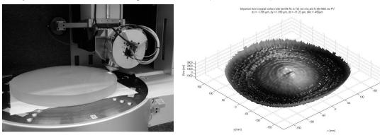
Fig. 7. Ø380 mm convex aspherical lens measurement (320 µm departure from base radius)
