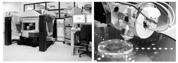
Fig. 3. The completed machine prototype and the inclined optical probe during measurement of a convex lens
