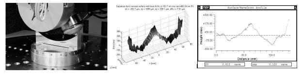
Fig. 8. Diamond turned freeform strip mirror (1 mm off-axis sphere), and NANOMEFOS and Zygo result
