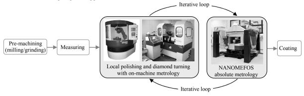
**Fig. 1.** Asphere and freeform production at TNO
