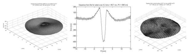
Fig. 9. Measurement of mid-spatials (spiral, centre defect and raster pattern from deterministic polishing)
