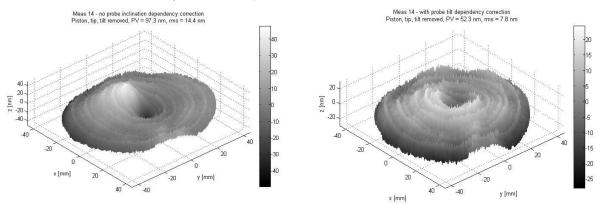
Fig. 6. Tilted flat measurement without (left) and with (right) the probe inclination dependency calibration
