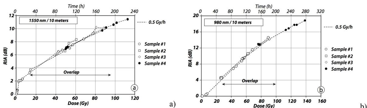
Fig. 5. Degradation kinetics at low-dose-rate, obtained from the switching dose rate experiments at 1550nm (a) and 980nm (b)
