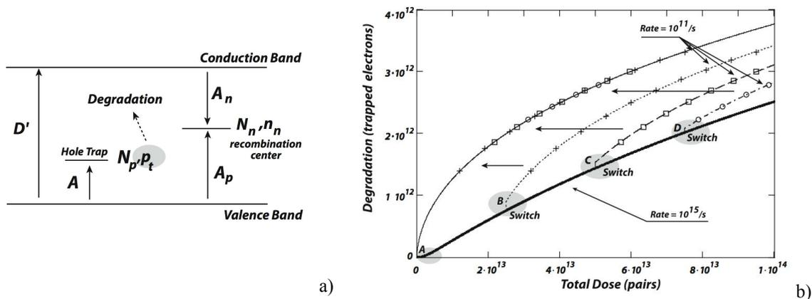
Fig. 2. a) Chen's Model b) Numerical Switching Dose-Rate Experiment built thanks to Chen's Model
