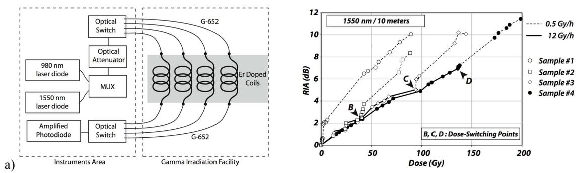
**Fig. 4.** a) Experimental "in-line" set-up. b) RIA versus the dose deposit for each of the 4 samples at 1550nm. Sample #1 was irradiated at low-dose-rate during the whole experiment. Samples #2, #3 and #4 were respectively switched from high-dose-rate to low-dose-rate at respectively points B, C and D.
