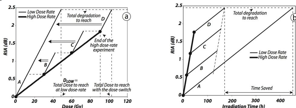
**Fig. 3.** Building the low-dose-rate degradation from switching-dose-rate experiments. a) switching dose-rate experiment vs the total dose. b) switching-dose-rate experiment vs the irradiation time.
