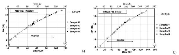
*Fig. 5.* Degradation kintetics at low-dose-rate, obtained from the switching dose rate experiments at 1550nm (a) and 980nm (b)
