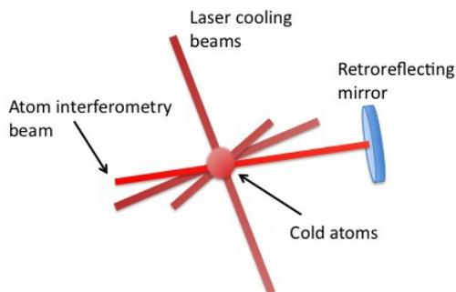
**Fig. 1.** Schematic view of the atom interferometer. The atoms are cooled down to  $10\ \mu\text{K}$ . The cooling beams are then turned off for the interferometric measurement, so that the cold atom cloud is in free fall. The retroreflecting mirror defines the phase reference of the laser ruler.
