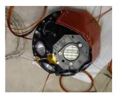
Figure 4. LRA equipped with its heater.
