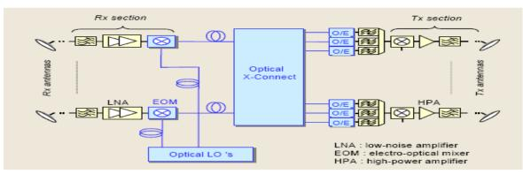
Fig. 1 : Flexible telecom repeater with microwave photonic cross-connect
