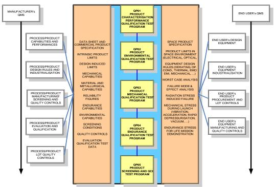
Figure 2: Qualification methodology proposed for development of high reliability optoelectronic products
