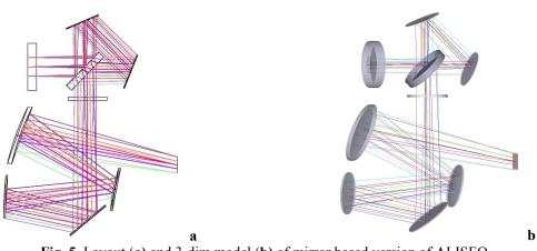
Fig. 5. Layout (a) and 3-dim model (b) of mirror based version of ALISEO
