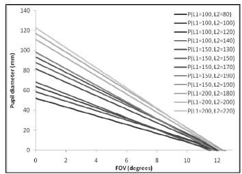
Fig. 2. Quasi-linear relation between FOV and entrance pupil for different interferometer arms lengths.
