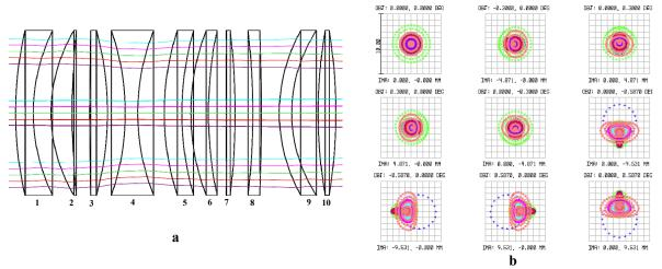
Fig. 3. Lens based focusing system (a). Spot radius diagram for the lens based system (b).
