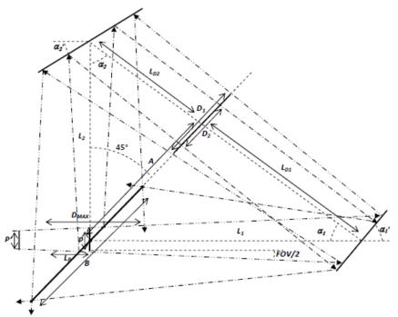
Fig. 1. ALISEO interferometer in Sagnac common path triangular configuration with its vignetting conditions.
