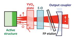
Experimental setup of the dual-frequency VECSEL
