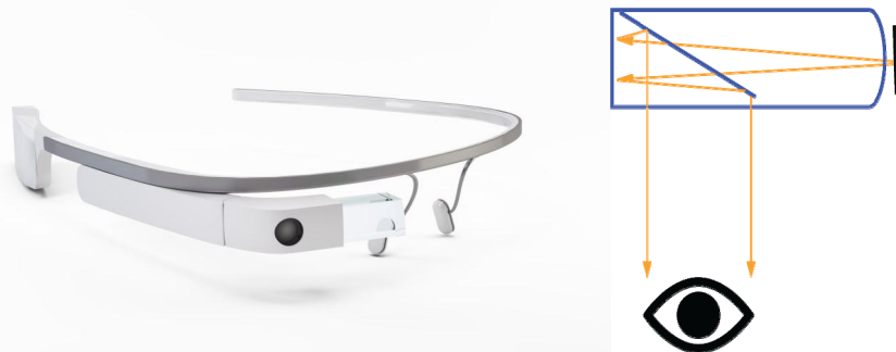
Figure 2. A photo of the Google glass, and its optical splitter cube (left); principle of light-guide architecture (right)
