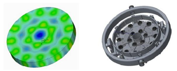
Figure 3. Left: Pseudo 3D view of a FEM simulation of the mounted primary mirror M1. Right: Gimbal mount, which was used within the simulation. The number of contact pads is 18. This is sufficient for a mirror diameter of  $d_{M1} = 400$  mm.
