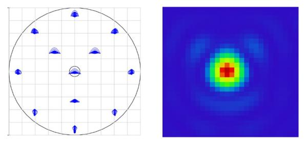
Figure 5. Left: Foci with a magnification of  $300 \times$  at a 36 mm x 36 mm detector plane. The radius of the systems Airy distribution is r01Airy = 5.4 µm. Right: intensity distribution of a PSF  $\neq$ in at (- 0.31, 0) ° deg with diffraction effects,  $\lambda = 550$  nm. The Strehl ratio of the point spread functions is  $\geq 0.8$ . Thus, the f/8 telescope is diffraction limited.
