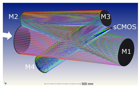
Figure 4. Optical path of the f/8 telescope ( $\emptyset$ M1 = 400 mm, tM1 = 50 mm, material: Zerodur, M1: parabolic mirror, M2: convex spherical mirror, M3: plane mirror, M4: concave spherical mirror. The entrance pupil of the system is placed at the left hand side.
