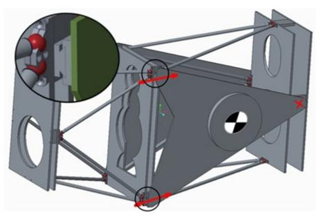
Figure 1. Pseudo 3D view of a telescope tube, which is based on carbon-fiber-reinforced-polymer (CFRP) tubes and plates. Originally this was designed for an f/7 system. The mounting axis, which provides the connection to the parallactic mounting fork, goes through the center of gravity.
