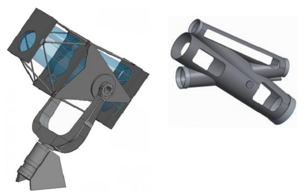
Figure 2. Left: Pseudo 3D view of a telescope tube in a parallactic mounting. Right: Pseudo 3D view onto a CFRP based monocoque telescope tube. The light gray metal rings indicate the compact mountings of the mirrors M1 to M4. The light enters the systems from the left hand side.
