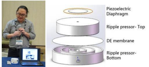
Figure 20: The demo of dielectric elastomer energy harvester autonomously primed by piezo- and tribo-electricity
