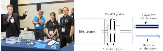
Figure 8: The demonstration of the Capacitive coupling as an underwater signal transmission interface
