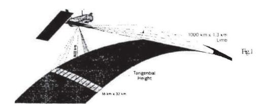
The long side of the Instantaneous Field of View is aligned parallel to the flight direction. It has a 1.8 deg angle corresponding to a width of 32 km in the flight direction at the subsatellite track. The maximum swath width of +/- 500 km ensure a global coverage with a maximum of three days at the equator and more rapidly at higher latitudes.
