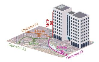
Figure 1. Application scenario for multi-operator PON transmission with MCF in-building network
