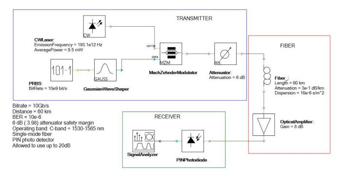
Figure 2. VPI Schematic diagram
