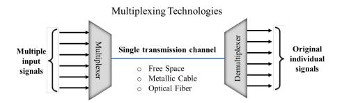
Figure 2. Concept of multiplexing/demultiplexing
