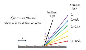
Figure 3. The incident light is diffracted into all primary wavelengths by a bulk-optic diffraction grating
