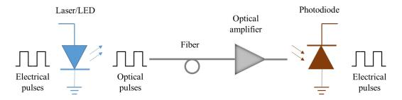
Figure 6. Schematic of optical communication system. The laser serves as the optical transmitter and the photodiode serves as the optical receiver.
