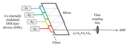
Figure 4. Schematic of a 4-channel CWDM multiplexer that combines four wavelengths and couples the multiplexed light signal into a single mode fiber (SMF).
