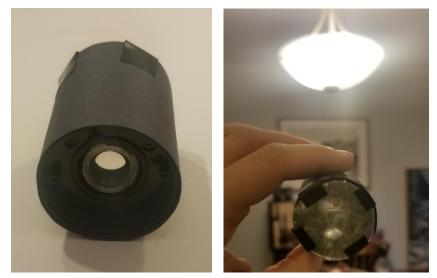
Figure 3. A simple construction paper tube camera obscura (left) with a wax paper "screen" for viewing the image (right).
