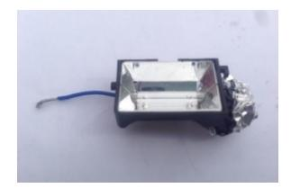
Figure 4. A static electricity detector using a camera's flash tube .
