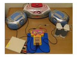
Figure 9. A simplified demonstration set for wavelength multiplied optical communication with a white-color LED.
