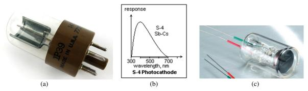
Figure 6. The side-window RCA/GE/Cetron 1P39 (929) vacuum phototube (a), its so-called S4 spectral response curve (b), and the front-end-window R-414 Hamamatsu phototube (c)
