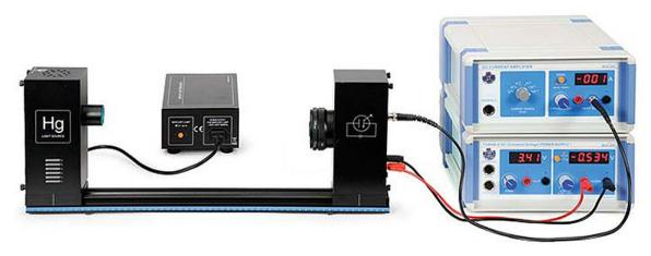
Figure 2. Photoelectric effect commercial experimental apparatus from PASCO [7]
