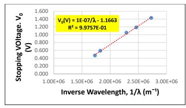
Figure 8. Stopping voltage as a function of inverse wavelength for the 1P39 photoelectric tube. The resulting value for Planck's constant is  $5.34 \times 10^{-34} J \cdot s$ , which is 18% off from accepted value. The work function of the cathode is 1.166 eV
