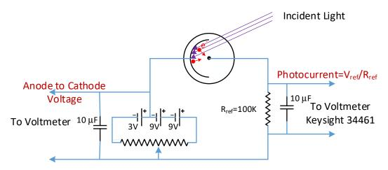
Figure 4. Circuit diagram of the photoelectric effect apparatus
