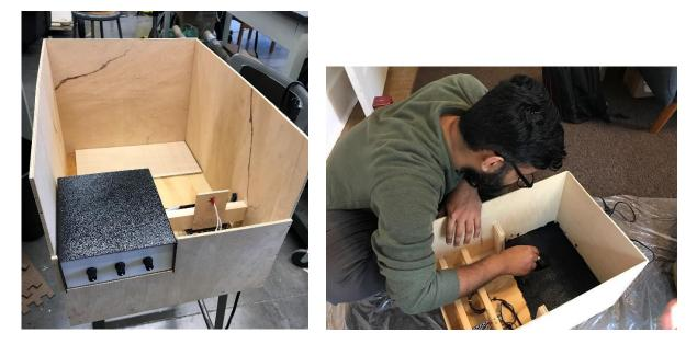
Figure 4. Unfinished color matching box and blackout painting. The unfinished color matching box (left) has tunable red, green, and blue LEDs and commercial light source mounted next to each other. A separator is placed between the sources to keep source spectra separate. To reduce the effect of wood spectral response on the light sources, the inside of the color matching box is painted black (right).
