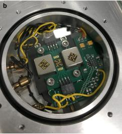
Figure 3. a) Schematic drawing of the experimental setup. b) Photograph of the detector chip sitting in-between two magnets inside a vacuum chamber.
