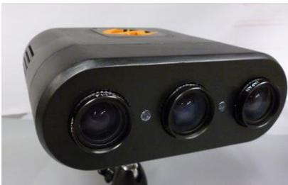
Figure 6: three sensor stereo system
