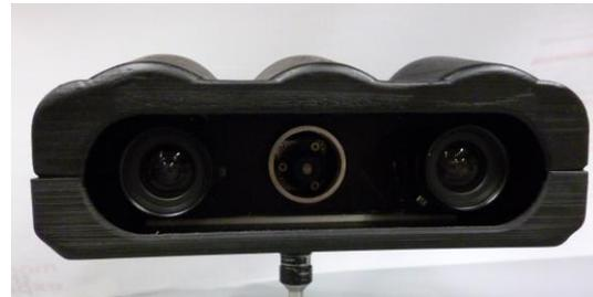
Figure 7: Stereo system with laser projector
