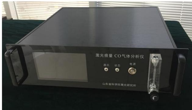
Figure 3. The engineering prototype of CO monitoring system.
