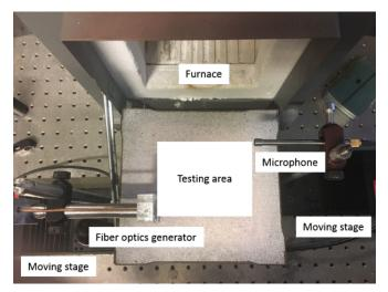
Figure 2. Experimental setup.
