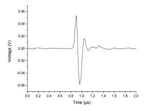
Figure 1. The ultrasonic signal generated by the fiber optic generator.
