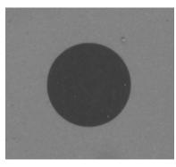
Figure 18. A cutout of the "Sample of optical calibration plate" of IMT Masken und Teilungen AG, incident light 99.6%, transmitted light 76.8%
