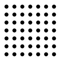
Figure 3. Point structure for a calibration target
