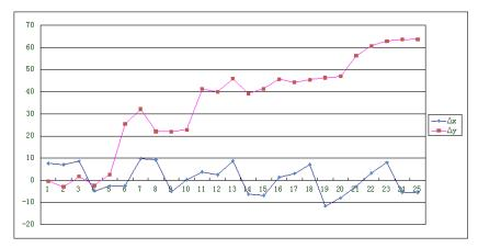
Figure 20. Position deviations [µm], foil "AVERY Zweckform Laser + Kopier-Folie", 1200 dpi, laser printer Lexmark Optra T610(MS)
