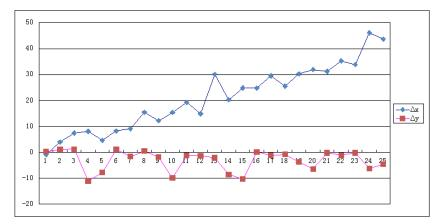
Figure 21. Position deviations [µm], photographic paper "HP Everyday Fotopapier", 600 dpi, laser printer Lexmark Optra T610(MS)
