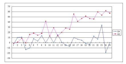
Figure 19. Position deviations [µm], normal copy paper, 1200 dpi, laser printer Lexmark Optra T610(MS)
