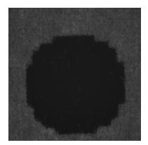
Figure 17. Visible dots of the printing process, normal copy paper, 72 dpi, inkjet printer HP K7100, incident light 52%, transmitted light 100%
