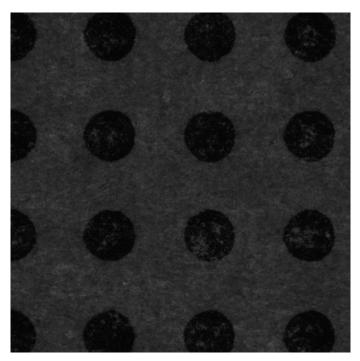
Figure 14. Normal copy paper, 1200 dpi, laser printer Lexmark Optra T610(MS), incident light 28.8%, transmitted light 100%
