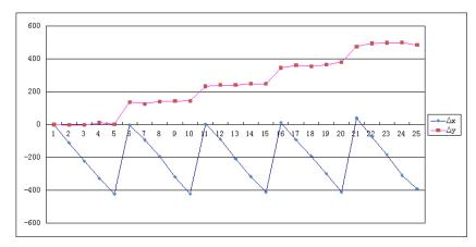
Figure 22. Position deviations [µm], normal copy paper, 72 dpi, inkjet printer HP K7100
