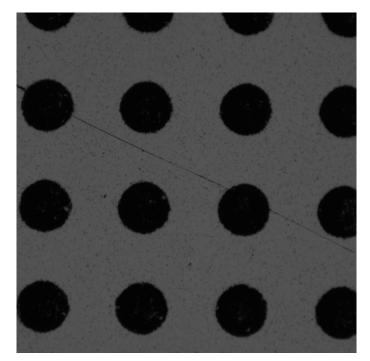
Figure 15. Foil "AVERY Zweckform Laser + Kopier-Folie", 1200 dpi, laser printer Lexmark Optra T610(MS), incident light 0%, transmitted light 16.8%
