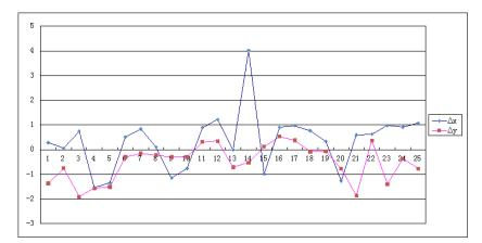
Figure 23. Position deviations [µm], "Sample of optical calibration plate" of IMT Masken und Teilungen AG
