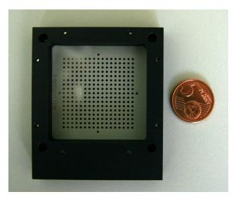
Figure 2. Chrome glass calibration target
