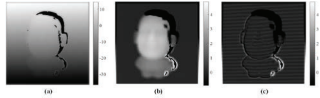
Figure 2. (a) The smoothed phase map by using Gaussian filter. (b) The smoothed phase map without carrier. (c) The difference between (a) and Fig. 1(b).
