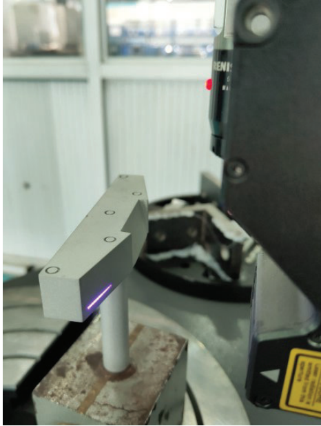
Figure 2. Contact probes and Line Laser sensor are measuring planar calibration blocks
