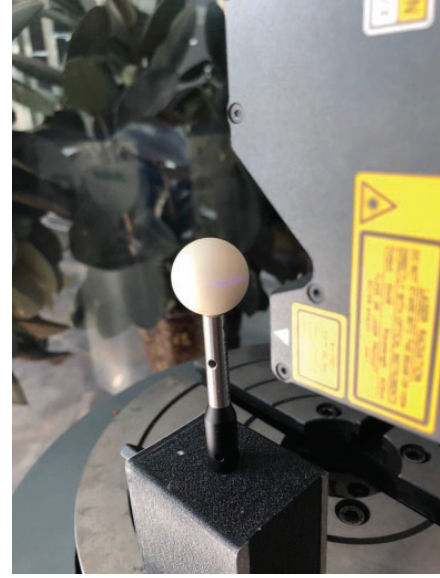
Figure 4. The line laser sensor is measuring the standard ball.
