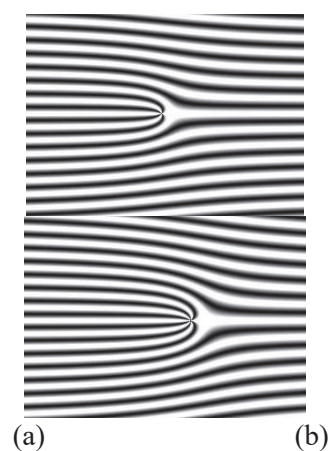
Fig. 9. Simulated (top) and experimental (bottom) interference fringes for optical vortices using reversal shearing interferometer: (a) m = 2 , (b) m = 3 , (c) m = 2 , (d) m = 3
