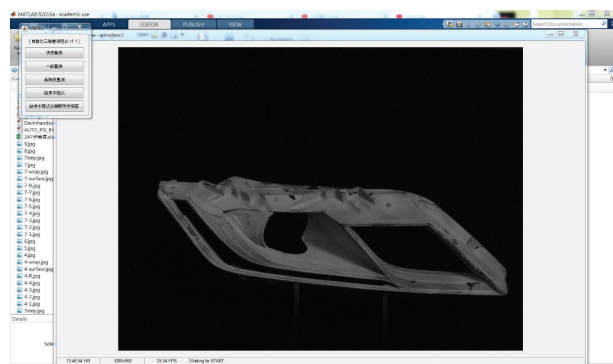
Figure 2. Operation interface of automatic digital fringe projection system.
