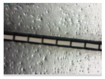
Figure 5: Microscope image of spectrometer entrance slit based stacked optical fibers. The rectangular fiber cores define the slit width in along-track direction (~100  $\mu$ m), and the spatial sampling distance in across-track direction. The scene heterogeneity is scrambled during propagation through the fiber (~20 mm). The spatial gaps between the fibers is due to the cladding around the cores, and serves to improve spatial co-registration. Courtesy CeramOptec.
