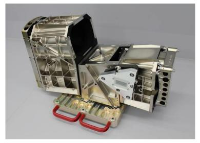
Figure 1. Optical system of the DESIS instrument. The telescope is on the left side, the spectrometer on the right. The light gray, triangular body is a detector dummy.
