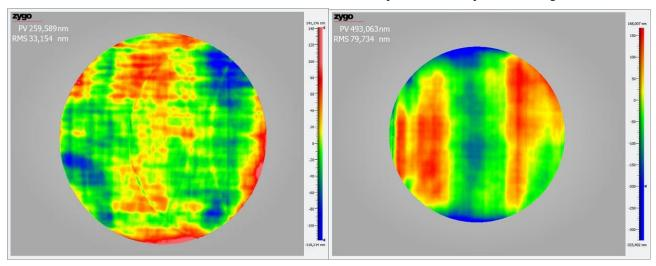
Figure 6. Measured wavefront errors of the TMA (left) and the spectrometer (right). The measurement position is in the center of the field of view.
