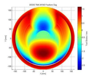
Figure 3. Map of the tool path used for the fabrication of the M1/M3 mirror module.
