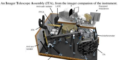
Figure 11.The IASI NG instrument with ATA & ITA telescope optics (Image Airbus)
