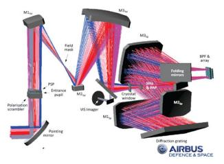
Figure 12. The MicroCarb instrument with 6 freeform optics (Image Airbus)
