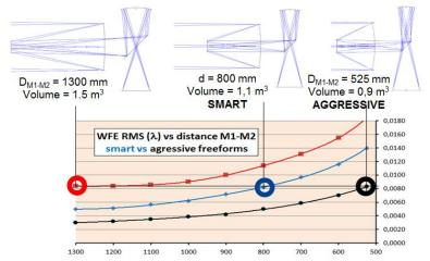
Figure 1. Pleiades telescope WFE RMS versus D<sub>M1-M2</sub> and type of freeform deformation introduction.
