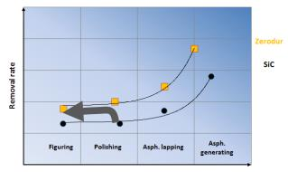
Achieved form error Figure 10.Process efficiency for Zerodur & SiC (arbitrary scale)
