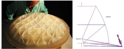
Figure 3. The MERLIN receiver's main mirror after lightweighting operations and optical sketch
