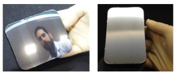
Figure 13. The MicroCarb first two mirrors prepared for R-SiC polishing layer deposition
