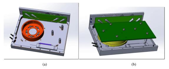
Figure 4: Booster box with (a) fiber spool and pump and photodiode board and (b) with fiber shield and controller board
