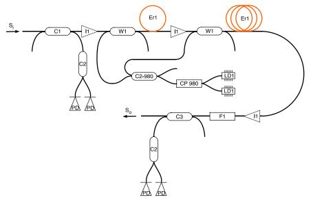
Figure 1: Schematic of the fiber pre-amplifier
