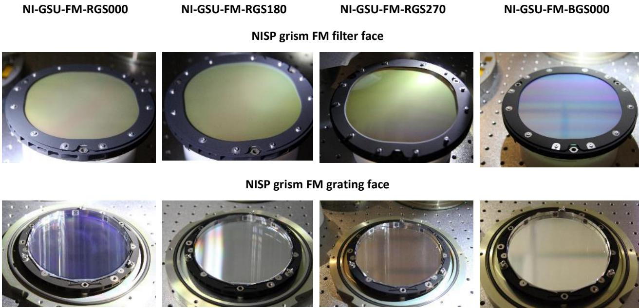
*Figure 3. The NISP grism flight models before delivery to NISP project. For each component, the filter and the grating surfaces are shown.*
