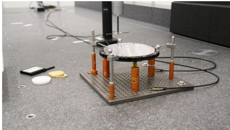
Figure 7. Picture of the FM RGS000 during its measurement on the CMM.
