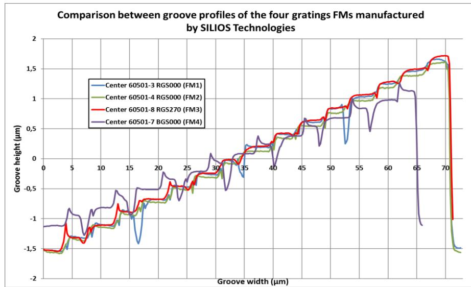
Figure 4: Grating groove profile measured on the four FM grisms.
