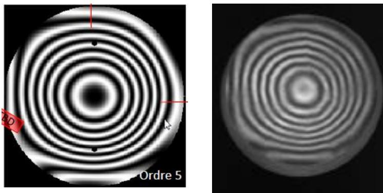
Figure 6. Theoretical interferogram for the grating of RGS270 in order 5 (left) compared to the measured interferogram of the FM RGS270 (right).
