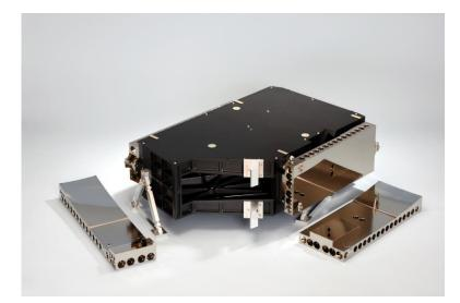
Fig. 3: Assembled telescope with two additional mirror modules M1M3 and M2M4
