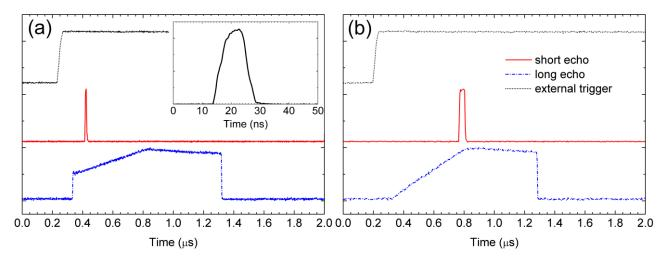
Figure 5. (a) Short pulse: 10 ns, shift 80 ns, long pulse: 1000 ns, initial amplitude p1 = 50%, flat part p2 = 50% of the pulse width, external trigger with 10 kHz repetition rate. Inset shows the short pulse: (b) Short pulse: 40 ns, shift 500 ns, long pulse: 1000 ns, initial amplitude p1 = 1%, flat part p2 = 50% of the pulse width, external trigger with 10 kHz repetition rate.
