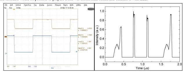
Figure 6. Left: Long pulse:  $270~\mu s$ , top – after logarithmic amplifier, bottom – direct measurement. Right: Example of an echo realization with multiple returns.
