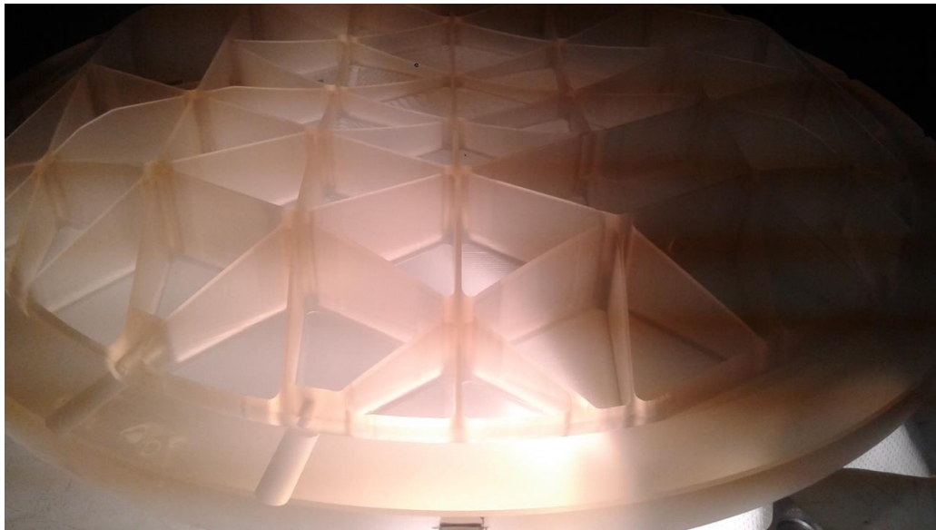
Figure 3-5 Photo of the M1RX QM mirror after acid etching, courtesy of Safran Reosc
