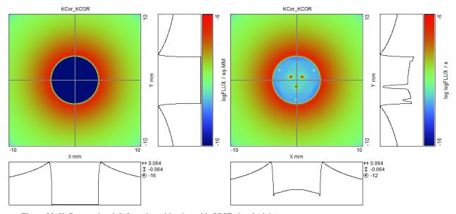
Figure 23. K-Corona signal (left) and combination with OPSE signal (right)
