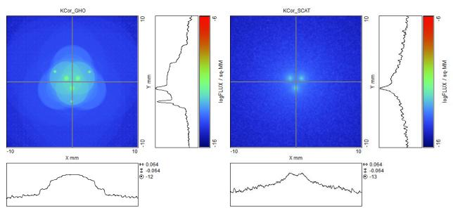
Figure 24. OPSE ghosts (left) and scattering (right) irradiance on the detector
