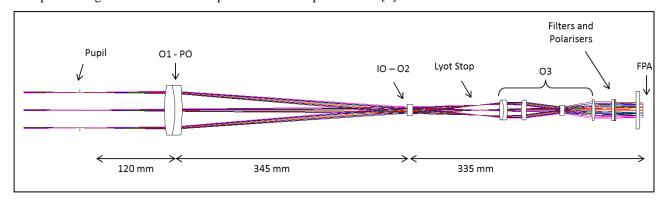
Figure 2 - Optical Model v15.2
