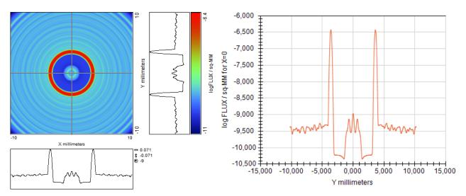
Figure 33. Final EO diffraction straylight irradiance on the detector after circular averaging
