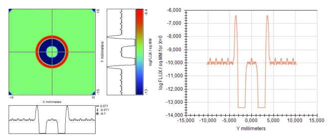
Figure 30. Ring of sources, ghosts from PO only, 501 rays on pupil grid
