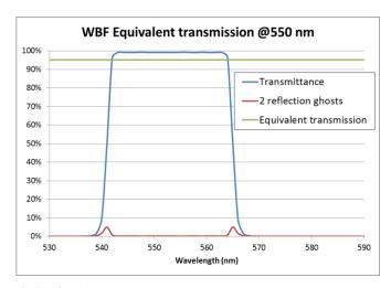
Figure 15. Equivalent transmission for the WBF
