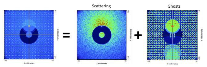
Figure 32. Ghosts and scattering from one source point on EO edge – 501x501 rays in pupil
