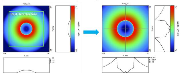
Figure 14. Coronal signal circular averaging, then crop to real detector size
