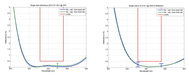
Figure 4 - Antireflection coating measurements (DM Lenses)
