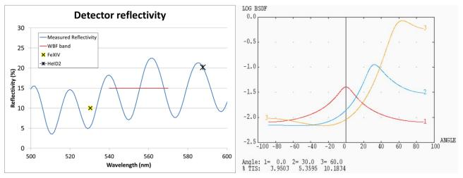
Figure 6 - Detector reflectivity measurement (left) and BSDF model of the anodized black coating (right)
