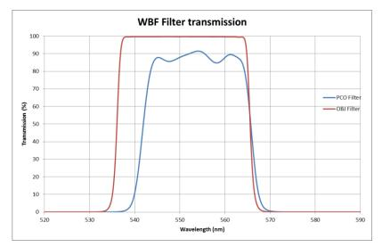
Figure 5 - Comparison of previous and new WBF transmission.
