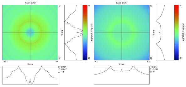
Figure 19. Ghosts (left) and Scattering detector irradiance (Right)
