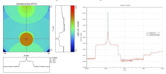
Figure 11. Ghosts distribution on the detector for a 1.29 RSun FoV (left) and transversal cut (right)
