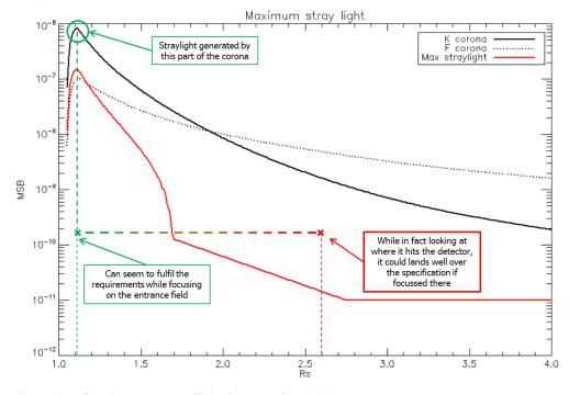
Figure 7 - Illustration of the instrument specificity in terms of straylight
