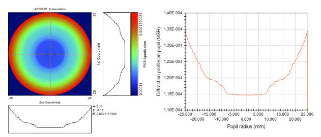
Figure 28. Pupil apodisation with diffraction profile
