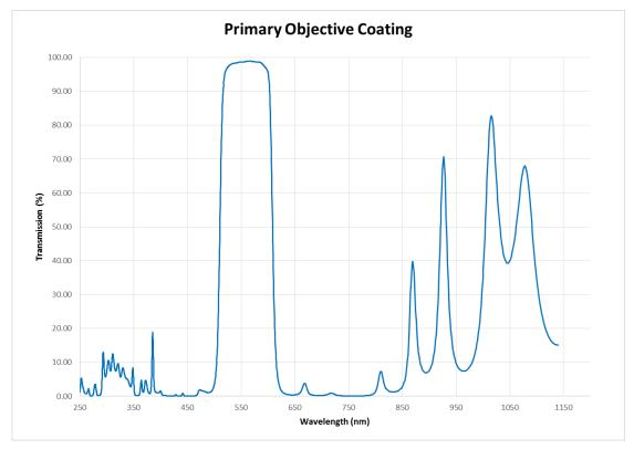
Figure 16. Primary Objective Coating transmission
