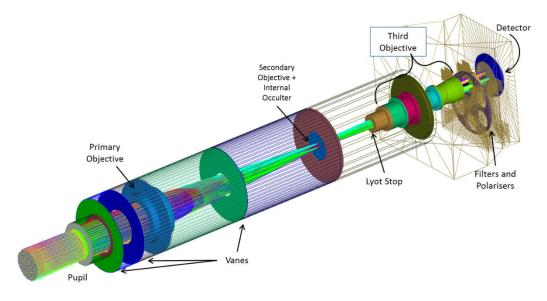
Figure 3 - Mechanical Model
