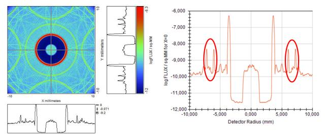
Figure 29. Ghosts and scattering from a ring on EO edge
