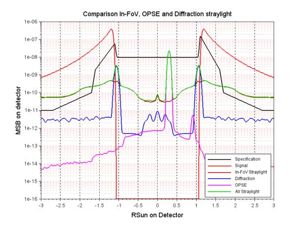
Figure 35. Final comparison of EO diffraction straylight with the KCorona, the in-FoV straylight and the specification
