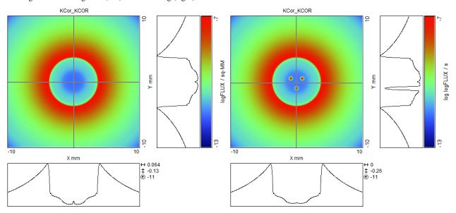
Figure 25. In-FoV Straylight and signal (Left), and combined with OPSE straylight and signal (right)
