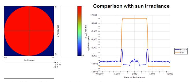
Figure 34. Sun source irradiance on pupil plane (left) and comparison on the detector plane (right)
