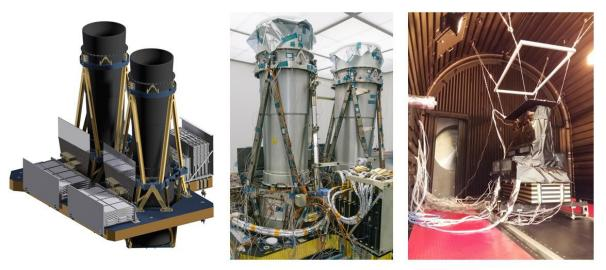
Figure 1. Ingenio/SEOSAT principal payload. Left: CAD model; center: flight model; right: flight model, covered with thermal blankets, during the thermal test campaign.
