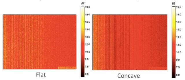
Figure 6 2D map of the RON for the flat sensor (left) and the concave one (right). The values are in numbers of electrons and are averaged in a 2\$\times\$2 pixels box.
