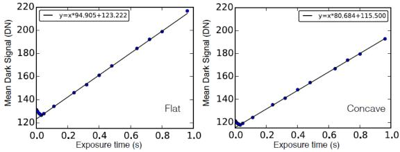
Figure 2 Mean dark exposure signal as function of exposure time. The black line is the fit to the data for exposure time larger than 0.048s. Left: data for the flat sensor. Right: data for the concave sensor
