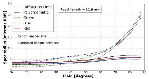
Figure 9. RMS spot radius size comparison for the two designs over the field of view. It demonstrates the obvious gain provided by the removal of the field flatteners.
