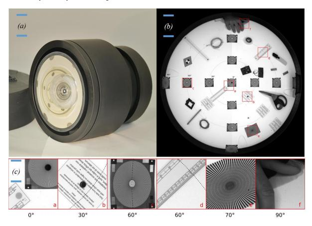
Figure 8 (a) picture of the as built 180deg FoV objective corresponding to figure 7 right. (b) 180deg picture taken with this objective combined with the convex sensor. (c) Detailed parts of the image showing the image quality over the field.
