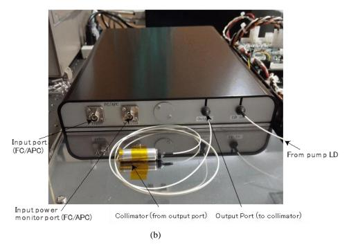
Fig. 2. The fabricated DP-DC-EYDFA: (a) inside and (b) outside.
