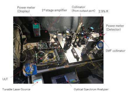
Fig. 4. Experimental evaluation system for the DP-DC-EYDFA.
