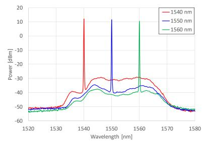
Fig. 7. Measured spectrum of the fabricated DP-DC-EYDFA between 1520 and 1580 nm (Wavelength of input signal: 1540, 1550, and 1560 nm, EYDF length: 5.5 m).
