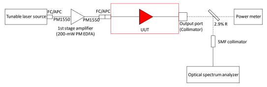
Fig. 3. Block diagram of experimental evaluation for the DP-DC-EYDFA.
