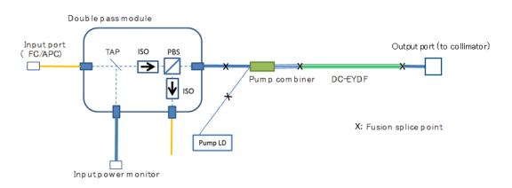
Fig. 5. Block diagram of the DC-EYDFA for SP evaluation.
