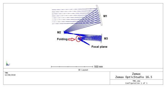
Figure 8. Layout of the TMA telescope
