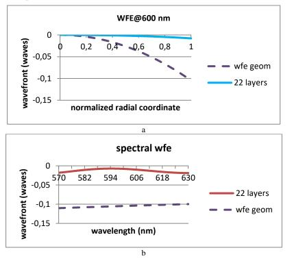
Figure 3. Wavefront of a 22-layer coating with high indices: a) radial and b) spectral profile with 2% thickness decrease.
