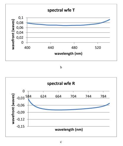
Figure 7. Transmittance and reflectance of a 18-layer coating: a) spectral intensity, b) transmitted wavefront, and c) reflected wavefront as function of wavelength with 2% of thickness non-uniformity.
