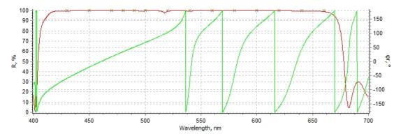
Figure 4. Reflected intensity (red) and phase (green) of a broadband mirror for the visible range, made of 46 layers of  $SiO_2$  and  $Ta_2O_5$  obtained combining two q.w. stacks, with a total thickness of 3.47  $\mu$ m.
