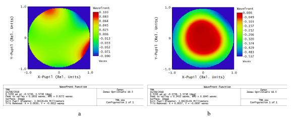
Figure 9. Wavefront map with a) the uniform broadband mirror and b) the non-uniform mirror, at the wavelength of 535 nm. The wavefront error, for the axial field of view, degrades from almost zero (0.03 waves rms) to almost 0.2 waves rms
