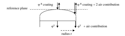
Figure 1. Coating with non-uniform thickness over the surface (radial symmetry).
