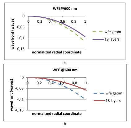
Figure 2. Wavefront of a) 19-layer and b) 18-layer high reflectance coating, compared to the geometrical wavefront (the radial coordinate equal to 1 corresponds to the minimum thickness reduced of 2%).
