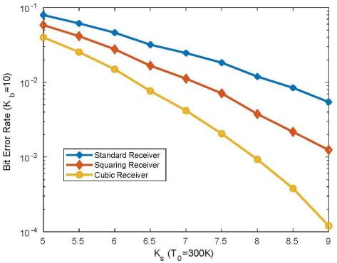
Fig. 6. Bit error rate of the standard, squaring, and cubic receivers. It is assumed that  $K_b = 10$ ,  $T_0 = 300K$ ,  $\bar{g} = 3500$ , F = 1. It is further assumed that the pointing error has caused 50% of the signal power impinge upon an adjacent detector.
