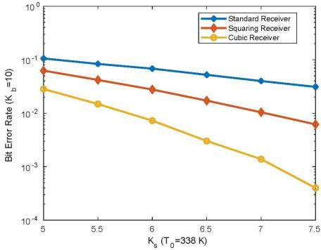
Fig. 4. Bit error rate of the standard, squaring, and cubic receivers. It is assumed that  $K_b = 10, T_0 = 338K, \bar{g} = 3500, F = 1$ .
