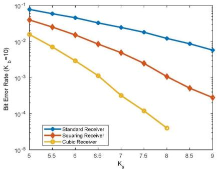
Fig. 2. Bit error rate of the standard, squaring, and cubic receivers. It is assumed that  $K_b = 10$ ,  $T_0 = 300K$ ,  $\bar{g} = 3500$ , F = 1.
