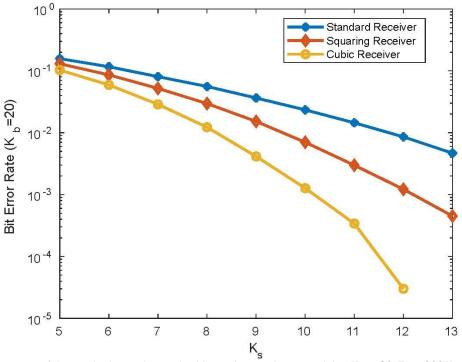
Fig. 3. Bit error rate of the standard, squaring, and cubic receivers. It is assumed that  $K_b = 20$ ,  $T_0 = 300K$ ,  $\bar{g} = 3500$ , F = 1.
