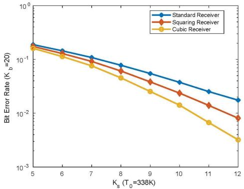
Fig. 7. Bit error rate of the standard, squaring, and cubic receivers. It is assumed that  $K_b = 20$ ,  $T_0 = 338K$ ,  $\bar{g} = 3500$ , F = 1. It is further assumed that the pointing error has caused 50% of the signal power impinge upon an adjacent detector.
