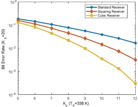
Fig. 5. Bit error rate of the standard, squaring, and cubic receivers. It is assumed that  $K_b = 20$ ,  $T_0 = 338K$ ,  $\bar{g} = 3500$ , F = 1.
