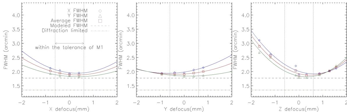
Figure 2 : Example of measured FWHM (on the array #2) as a function of defocusing distance along the X axis (right), Y axis (center), Z axis (left). For each axis, a defocus of 0mm corresponds to the best theoretical focus.
