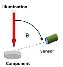
Figure 5: Configuration for the measurement of a BRDF pattern
